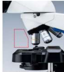
Inward-facing revolving nosepiece
